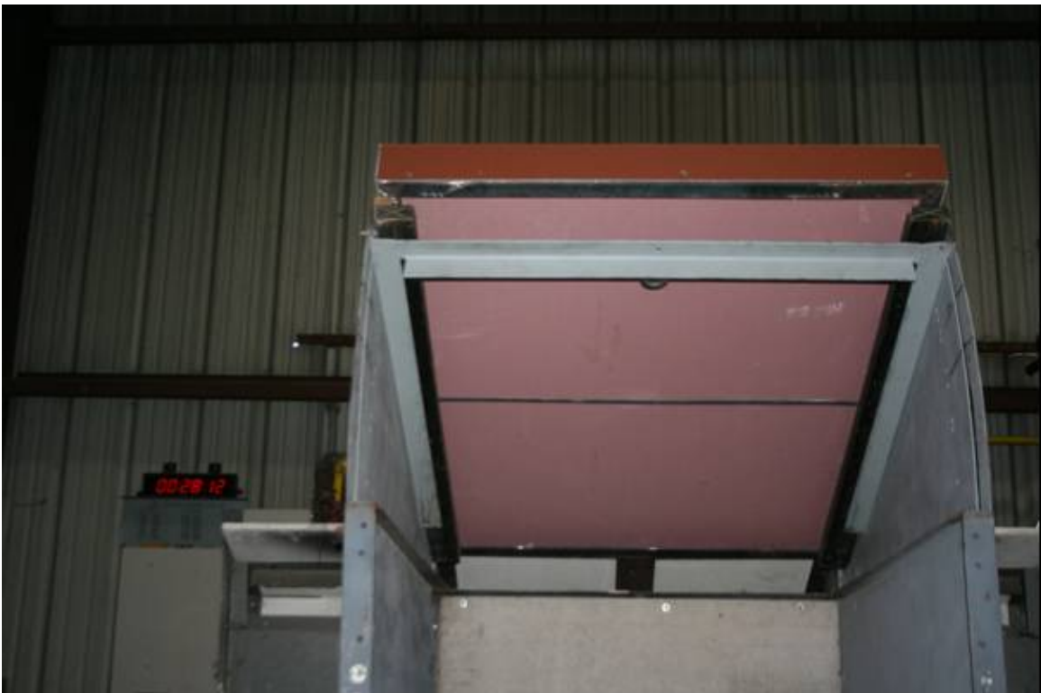
Figure B-8. Test ID BB-2. Underside of Test Sample at End of Test.
