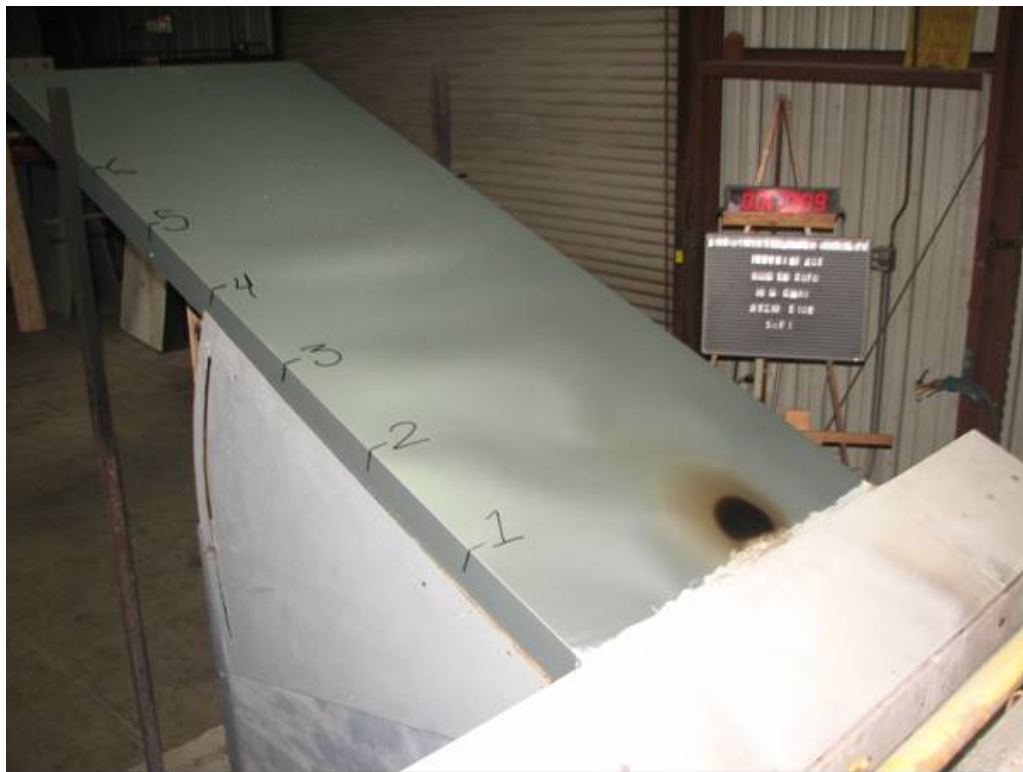
Figure B-4. Test ID SoF-1. Test Sample at End of Fire Exposure.
